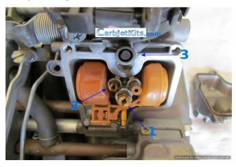
To the far left is the Pilot Screw (2). The Main Jet (1) is in the center and is screwed in the jet holder. Remove pilot jet and main jet using a flat screw driver. The jet holder often comes out with the main jet.
