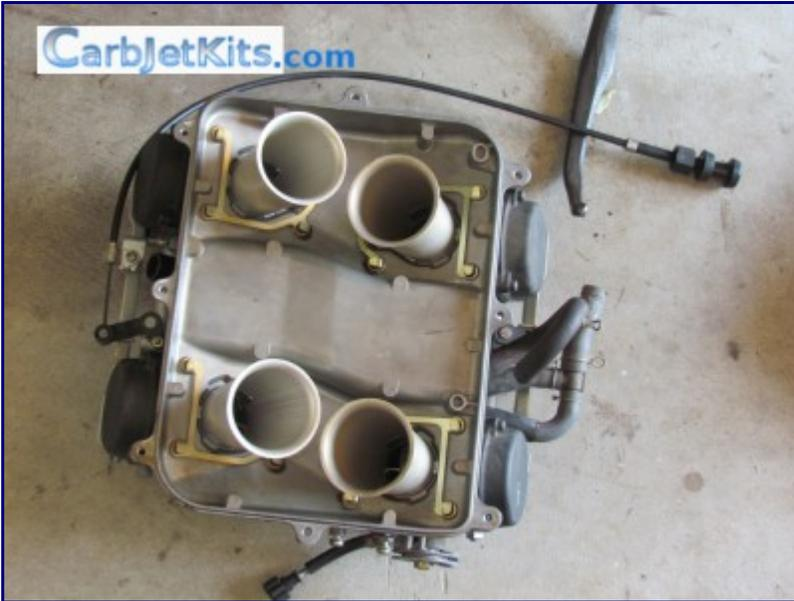
Before we start please make sure you drained all fuel from the carburetors by opening the drainscrews on the carburetor bowls. Do not turn your carburetors upside down to drain the fuel. do not smoke and keep away from open flames.
