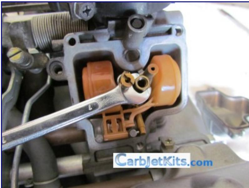
Remove the old main jet using a flat screwdriver and a wrench.
